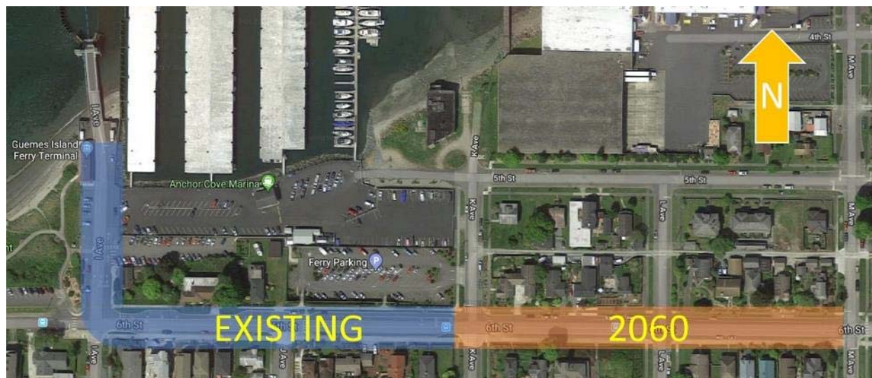
Figure 13 Existing Anacortes terminal delineated queue lane (blue) and additional length required to accommodate 2060 forecast (orange)
