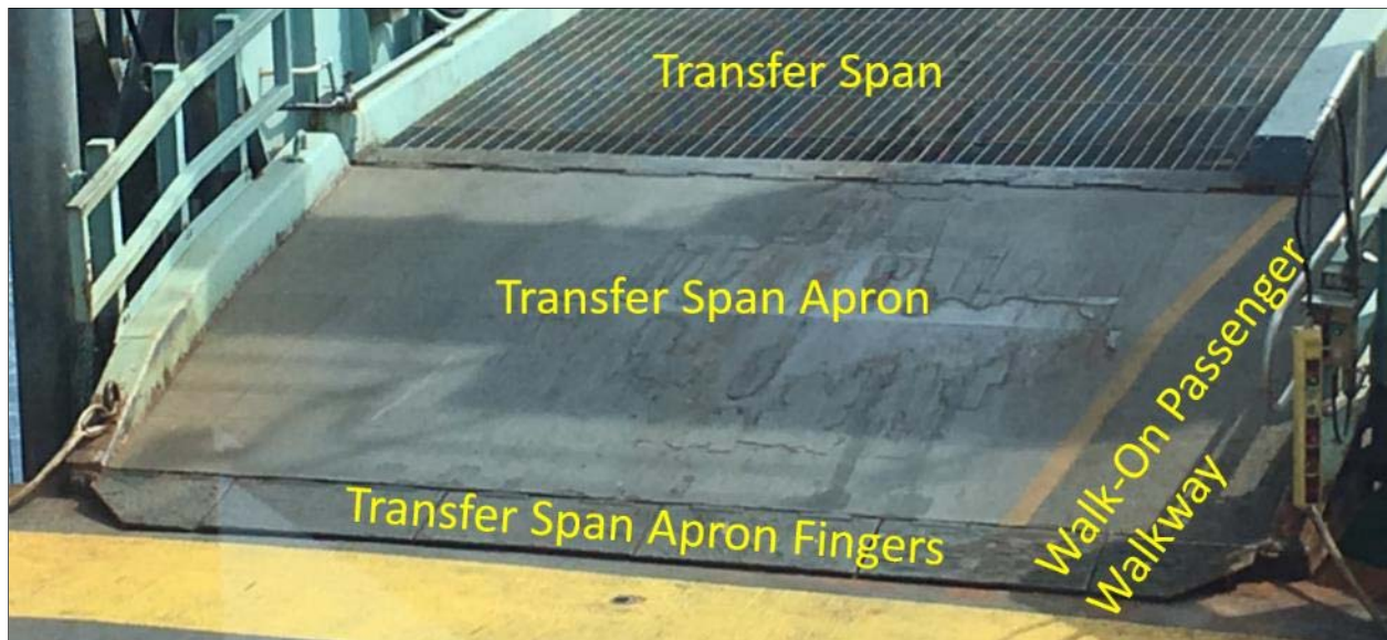
Figure 1 Transfer span components
